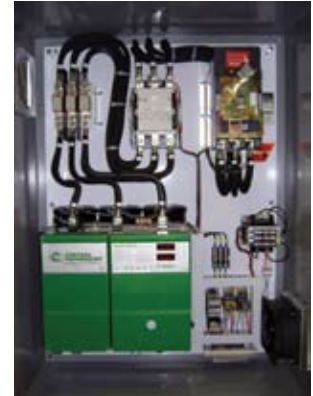
MentorPak PN: DEN4255AN1A0-E Nema -12 (PPBF), Ventilated Encl., 150 hp, 460 VAC, Non-Regen, Circuit Breaker, AC Contactor, BMS
