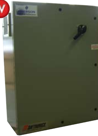
MentorPak PN: DEN4255AN1A0-E Nema -12 (PPBF), Ventilated Encl., 150 hp, 460 VAC, Non-Regen, Circuit Breaker, AC Contactor, BMS
